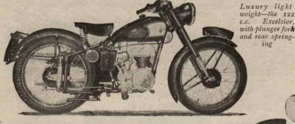
Transfer ports are on both left and right of each cylinder. The separate heads are light-alloy castings. The exhaust pipes lead into a single large silencer, mounted alongside the left-hand chainstay.
