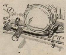
New arrangement of the Ariel Four brake pedal and exhaust pipe to enable greater travel of the pedal
