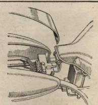
A junction box is neatly arranged at the rear of the tunnel in the Tandon tank
