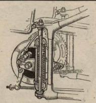
Detail construction of the Excelsior rear-wheel springing
