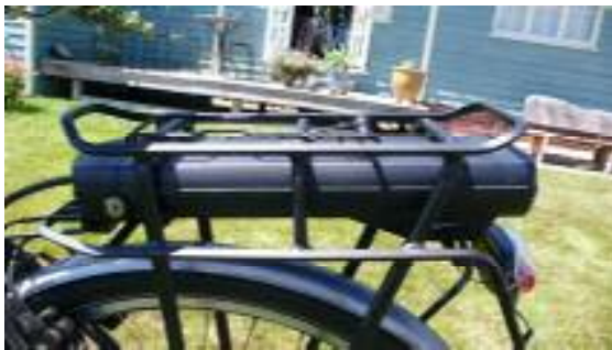
The Lithium battery location.
