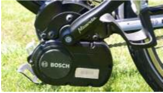
The crank mounted power plant.
