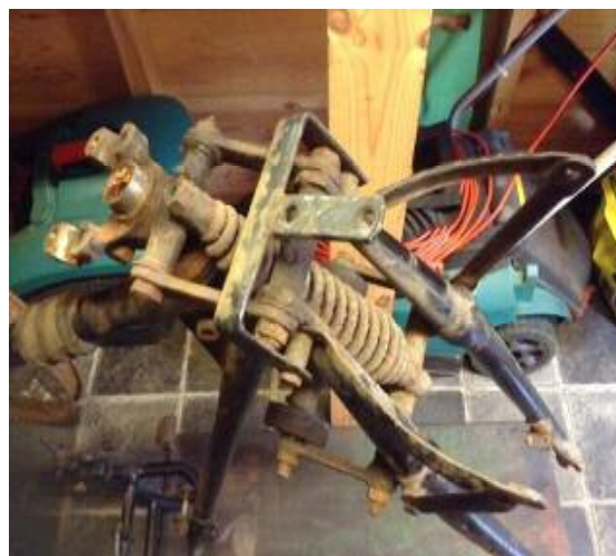
The completely seized up front suspension assembly.
