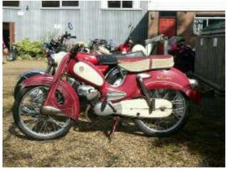
This Victoria Vicky 117 was one of the rarer mopeds seen on the Radar Run. It's a 3-speed machine with leading-link front suspension. Maybe its rarity is due to the fact that the 117 was only imported to the UK between June 1963 and October 1964.
