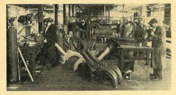
Left: Welding being carried out on frames and tanks.
