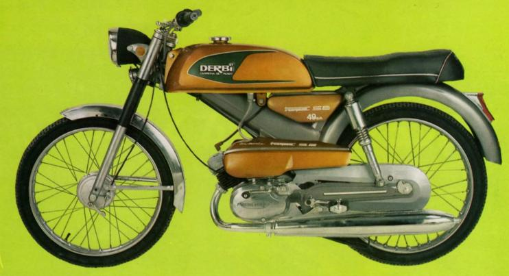
High performance 2-stroke engine built by Derbi 38 mm, bore 44 mm, stroke 48.7 G.C.
