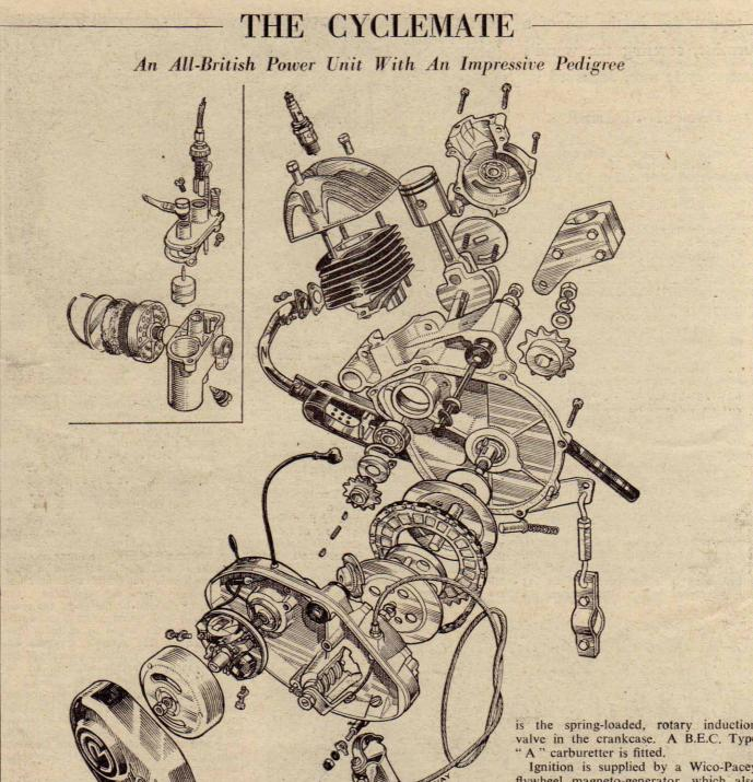
DIRECT descendant of the famous A Cyclemaster "engine-in-the-wheel" power unit, the Cyclemate is British-built throughout, and is the smallest moped unit available to-day. With bore and
