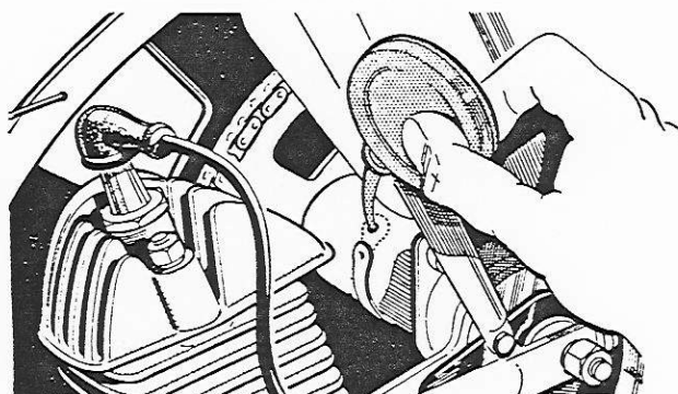
The lubrication hole in the New Eadie Coaster Hub.
