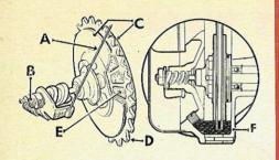
The Cyclemaster engine is fitted with a clutch, enabling the rider to keep the engine running at traffic stops. A. Clutch cable to handlebar lever. B. Adjusting screw. C. Clutch plates. D. Main drive sprocket. E. Clutch corks. F. Oil chamber.
