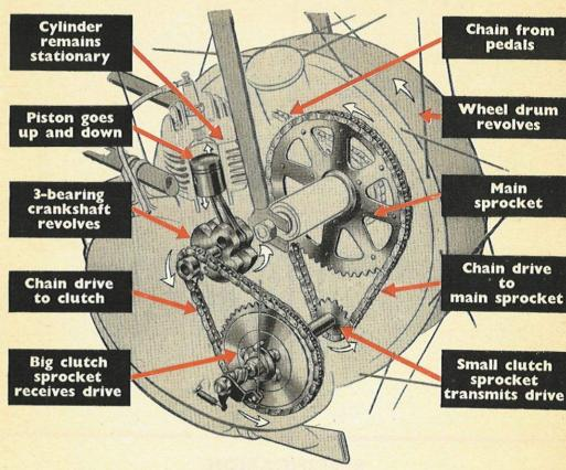
This much simplified diagram explains how the Cyclemaster engine works, but cannot show the many engineering features which make it the only sensible form of power-assisted cycling.
