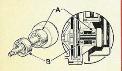
There are two ball bearings on the clutch shaft, A and B in this illustration. The bearing A also takes up the end thrust of the shaft.
