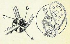
Smooth, vibrationless running and long life are also ensured by the cushioned drive. A and C are metal segments. B rubber cushions which give perfect smoothness.
