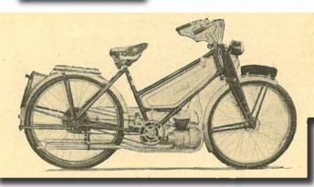
The Cyc-Auto, with its low engine mounting and worm primary drive, is unique among autocycles
