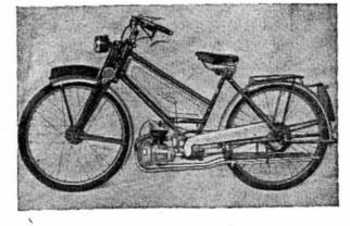
guards. A built-on carrier is provided and the twin plated exhaust systems extend right back to rear of the machine so that no petrol messiness is experienced at all.
