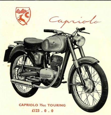
Single cylinder, 4 stroke, O.H.V. cam shaft, flywheel magneto, roller bearing throughout engine, 4 speed foot change gearbox.
