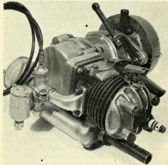
*The original Busy Bee 50 cc engine (1 $\frac{5}{8}$  in. bore  $\times$  1 $\frac{1}{2}$  in. stroke).*
