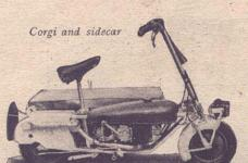
FOR next year, the Brockhouse Corgi is being continued unchanged. Rigid-chassis and banking sidecarriers are available, as well as conversion kits for fitting a two-speed foot-operated Albion gear box and a Druid telescopic fork. The banking sidecarrier is a Feridax project; and the gear box and fork conversions have been developed by Aston Bros., of Coventry, in conjunction with Albions, Druids and Jack Oldings.
