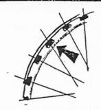
Remove the rear wheel from the Bicycle and attach the driving rim to the spokes on the side of the wheel opposite to the chain sprocket, and lightly clause in position.
