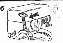
Loop the driving belt round the motor pulley and the wheel rim and adjust for tension. There are two slots provided in the rear motor bracket for this purpose, and the two screws must be tightened when all slackness in the belt has been taken up, and a small amount of spring pressure will keep it tast.
