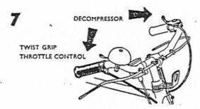
Fit the handle bar controls. The twist-grip throttle control must be adjusted so that the engine stops when the control is turned to the shut position.
