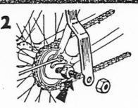
Remove the existing rear spindle nots which will not be required. Fit the extension bolts supplied with the motor. These are hollow to accommodate a 3-speed control if one is fitted. 3
