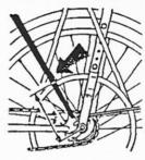
can best be done by making a chalk mark on the bottom stay tube about 7½ inches from the hub spindle. Rotate the wheel and gently tap the rim notil it runs true in relation to the chalk mark, tighten up the clamp screws all round the rim.
