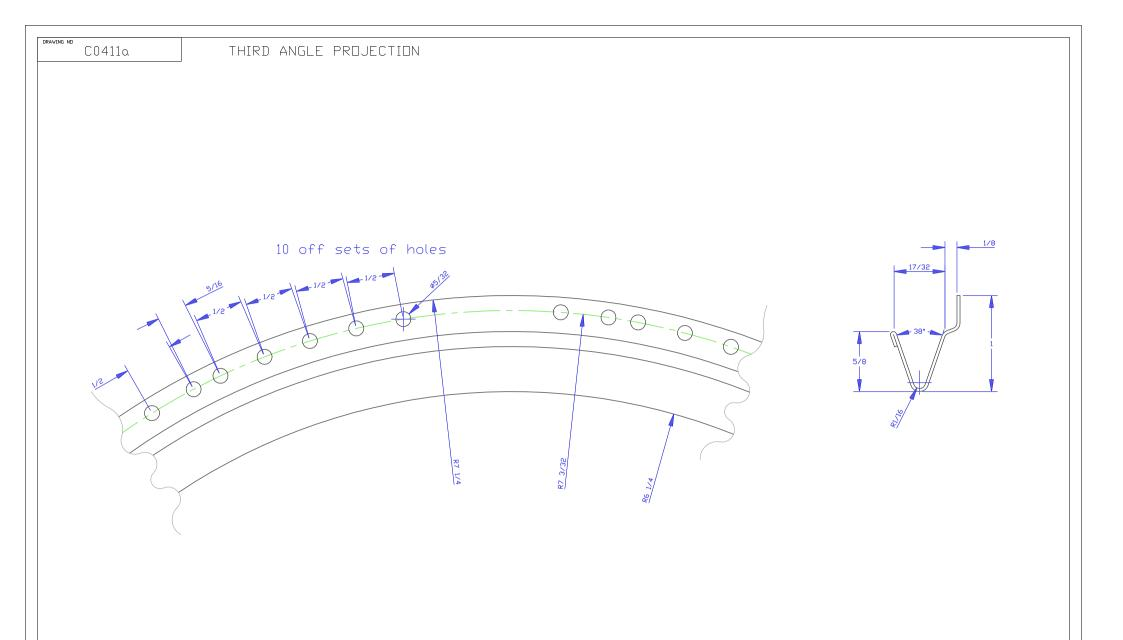
Original drilling shown for 40 spoke wheels Modern 36 spoke wheels will need 9 sets of holes Material: 20swg M/S
