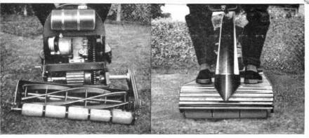
LAWNRIDER DOES AWAY WITH THE GARDEN ROLLER Full-weigh of machine plus full weight of drive —directly applied.
