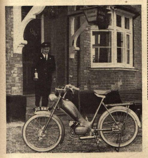
THERE'S plenty of beef behind the Berini M.21, the fascinating single-speed Dutch moped which has formed my staple means of transport for the past week or so. It is an elegant machine this, with a sturdy heart. No sluggard either, for its maximum speed of 29 m.p.h. can be reached easily on any level road, and a 25 m.p.h. cruise is not beyond its capabilities.
