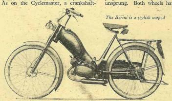
are fitted with 2in white-walled tyres and incorporate hub brakes; that at the rear is of back-pedalling type. Interesting features of the controls are a trigger to hold the clutch out of engagement when manœuvring the machine by hand, and a device which automatically opens the starting choke when the throttle is opened.
