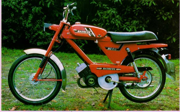
The handling of the machine demands a great deal of care, as the steering is very light and, perhaps, the forks are mounted too near the vertical plane. This is all very well when manoeuvring through traffic but, when travelling at more than a walking pace, the whole feels quite unstable and twitchy. one has to remember is to
