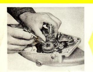
Apply jointing compound evenly to the edge of one crankcase and allow it to become "tacky". Insert the
