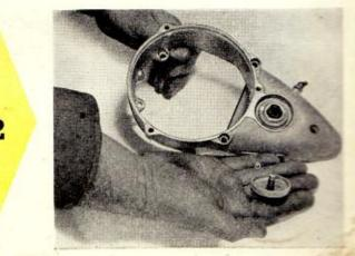
Fit the selector mechanism to the right-hand side half-case so that the spring loaded plunger (A) engages in the deepest notch on the quadrant. This is second
