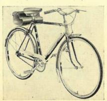
another bright feature is the red anodized bottle on the down tube. Polished alloy Continental mudguards and the four bright seat bands provide a shining contrast to the main frame colours of black or zircon blue. Campagnolo gears are fitted and with top-tube brake clips, and pump in front of the seat-tube, this will be a showpiece of the Italian trend allied to best British workmanship. Very competitive, too, is the price, £26 19s. 6d.
