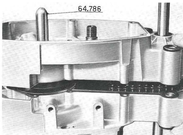
— With the exception of the Bosch flywheel, insert the distance piece under the stator plate, fit the plate so that the scribe mark «S» previously made is in line, tighten the mounting screws «V1».
