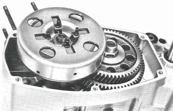
— Hold the 2nd speed housing «C» with the tool 64766 and tighten the nut to 3÷4 kpm (in.lb. 0,168÷0,224) with the torque wrench.
