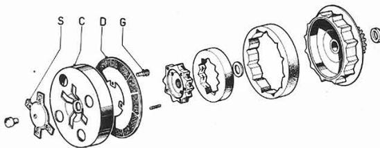
— When at the disc «D», place the 4 rubbers «G» in the corresponding holes. The rubbers ends should face towards the outer side of the engine and the thicker lined face of the disc towards the inner side.
