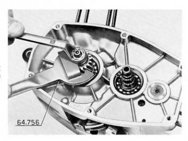
Hold the gear with the tool 64.757 operate its centre screw and slide the gear from the crankshaft with a 19 mm (.748") wrench.
