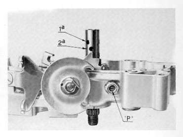
Place the balls in the respective holes on the secondary shaft and hold them in place with some grease.
