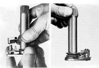
Slide the selector group into the right hand crankca-se, lightly tighten the 2 hexagonal screws.
