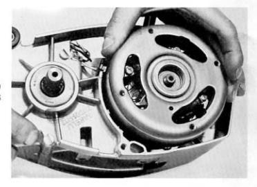
— Rotate the flywheel by hand in the clockwise direction until the points gap is in the widest position. At this instant check the gap with a feeler gauge, resetting if necessary to 0,35÷0,45 mm (.014"÷.018") Check the timing, which is correctly set when the points begin to open at 23° B.T.D.C. (for 5 speed only: 26° B.T.D.C.) (see owner's manual).
