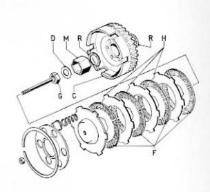
Place on the primary shaft the shim washer «R», the clutch housing «C», the other shim washer «R», fit the clutch hub «M», the washer «D» and the nut «G». Hold the clutch hub with a 30 mm socket and tighten the nut «G» to 4,5÷5 kpm (in.lb. 0,252÷0,280) with the torque wrench.
