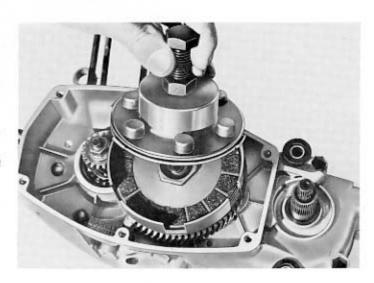
With a 10 mm (.393") socket and screwdriver adjust the play (6÷8 mm) (.236"÷.314") of the clutch discs control rod.
