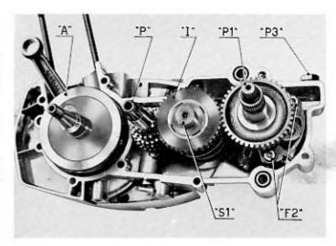
Secure in a vice the secondary shaft of the 5 speed engine, draw back and slide off the slider taking care not to lose the springs and locating balls.
