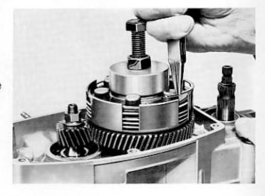
Hold the clutch hub with a 30 mm (1.181") wrench, unscrew the lock nut with a 17 mm (.669") socket, slide the washers, the nut and the hexagonal body.
