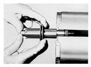
Before starting to assemble the unit, carefully clean and slightly oil all the parts.
