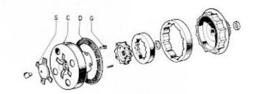
When at the disc «D», place the 4 rubbers «G» in the correspondig holes. The rubbers ends should face towards the outer side of the engine and the thicker lined face of the disc towards the inner side.
