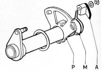
Once the group is assembled, the spring «M» should be engaged with the plate «P» and anchor «A» as illustrated.
