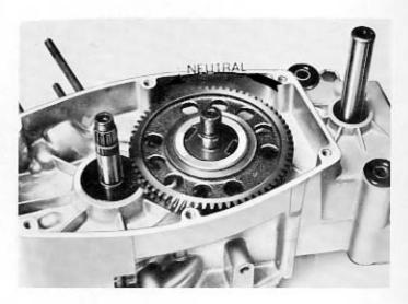
With the tool 64781 and torque wrench tighten to 8÷8,5 kpm (in.lb. 0,448÷0,476) the nut fixing the gears on the primary shaft.
