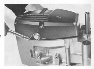
Remove the left sidecover and its gasket by taking out the six screws that hold it to the crankcase.
