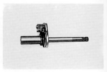
Fit the gearchange lever «C» sliding the control fork into the sleeve «D», then place the sleeve in place using the tool 64785.
