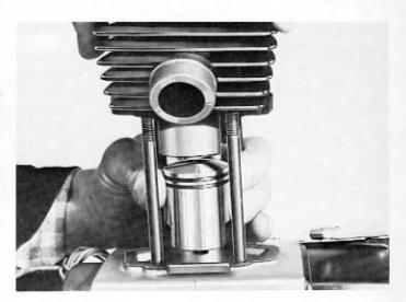
— Check that the top of the cylinder and the face of the head are clean and undamaged. Fit the head over the studs and place the 4 washers and nuts on the studs. Tighten the nuts gradually in a cross pattern. The final torque should be 1,5÷1,8 kpm (in.lb. 0,084÷0,10). Refit the spark plug.
