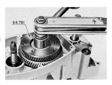
Remove the 2nd speed gear and then the 1st', while holding the catches with the tool 64784.
