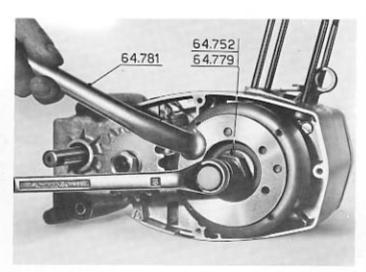
— Make a scriber mark «S» across the bottom of the stator plate and the crankcase in order to facilitate re-timing on assembly. Remove the screws «V1» holding the stator plate to the crankcase. Remove the Woodruff key from the crankshaft.
