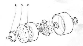
Before mounting the plate «S», the elastic body «C» and the circlip «A», with the tool 64767 and torque wrench tighten to 3÷3,5 kpm (in.lb. 0,168÷0,196) the nut fixing the clutch hub to the crankshaft.
