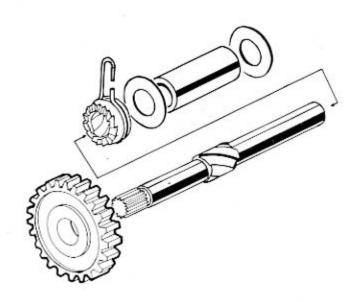
Slide the crankshaft, lightly tapping it with a mallet.
