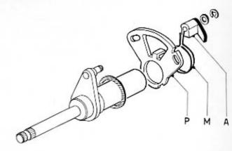
To have the group assembled correctly, the spring «M» should be engaged with the plate «P» and the anchor «A» as per illustration.
