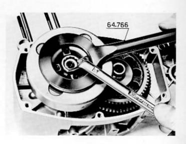
Take the assembly of two clutches complete with gears and slide it from the crankshaft.
