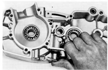
— Insert the selector group in the right hand crankcase, making sure that the grub screw «F» on the lever «C» is properly seated in the slide of the selector drum «G». Tighten the 2 hexagonal screws «V». Then tighten the screw «P3» and nut. The more the screw is tight, the more accurate is the speed passage.
