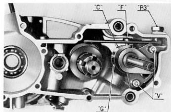
— Using the tool 64777, operate the gearchange lever to drive the sleeve nibs «N» in the 2nd and then in the 3rd speed position, and make sure that the slider sideway swivel (both up and down) is steady. To regulate this, rotate the gear selector quadrant «D» in the appropriate direction until adjustment is got, then tighten the 2 screws «V».
