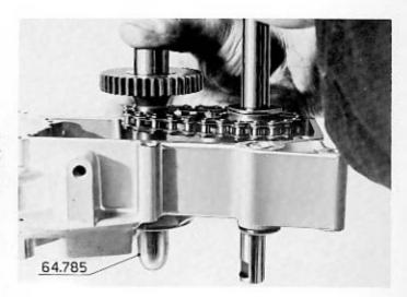
Insert the crankshaft into the crankcase, lightly tapping it with a mallet.
