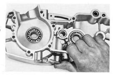
Fit the gearchange lever «C» slipping the gears operating slider into the sleeve «D» placed on the secondary shaft.
