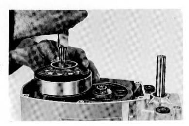
Using the tool 64767 and a 17 mm (.669") socket remove the nut locking the clutch hub. Then slide the clutch hub and housing from the crankshaft.
