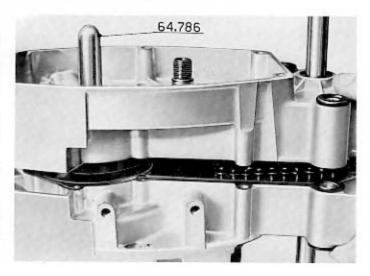
With the exception of the Bosch flywheel, insert the distance piece under the stator plate, fit the plate so that the scriber mark «S» previously made is in line, tighten the mounting screws «V1».
