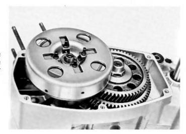
Hold the 2nd speed housing «C» with the tool 64766 and tighten the nut to 3÷4 kpm (in.lb. 0,168÷0,224) with the torque wrench.
