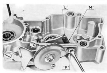
Slide the secondary shaft in the support and then in the bearing, using the tool 64785.
