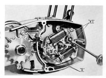
Fit the woodruff key in position on the crankshaft, slip the flywheel and rotate it until it is felt that the key is correctly seated.
