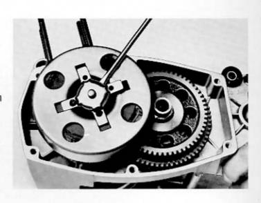
Holding the clutch body with the tool 64766, use a 17 mm (.669") socket to unscrew the nut, then remove the washer.
