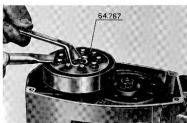
Holding the gear with the tool 64781, unscrew the nut with a 17 mm (.669") socket.
