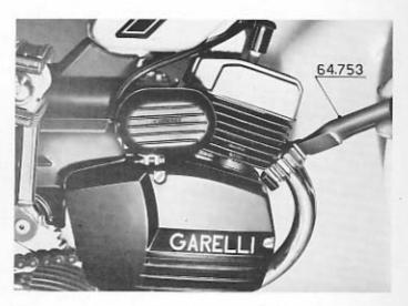
Disconnect the starting cable using a 17 mm (.669") open end wrench as illustrated.
