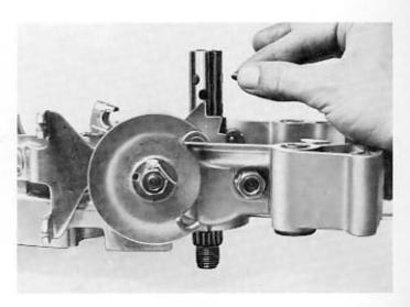
Mount the primary shaft and then the gears on the secondary shaft. Make sure that the toothings are in line.
