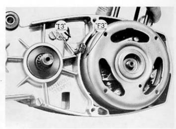
When satisfied that the gap is set correctly, fit the washer and tighten the fastening nut, using the tool 64781 and the 14 mm (.551") socket previously used when dismantling.
