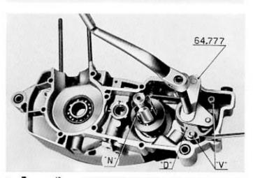
Slide the crankshaft «A» in the right hand crankcase and the primary shaft «P» in place.
