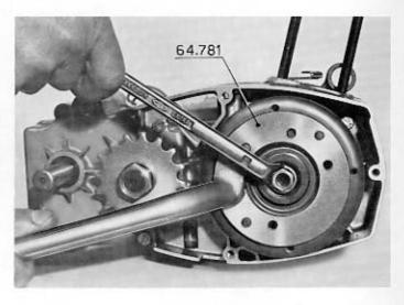
Fit the chain gear and the two shim washers on the secondary shaft, using the tool 64753 and a torque wrench tighten the nut to 6÷ 6,5 kpm. (in. lb. 0,336÷0,364).
