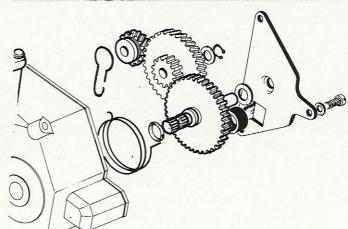
When refitting the starting assy., make sure that the return spring «M» is correctly in place as illustrated. (this operation also applies to the single speed kickstarter models).
