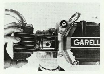
— Check that the top of the cylinder and the face of the head are clean and undamaged. Fit the gasket and the head over the studs and place the 4 washers and nuts on the studs. Tighten the nuts gradually in a cross pattern.
