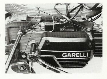
Remove the 4 nuts holding the cylinder head using one 11 mm (.433") box spanner. Lift the head and the barrel over the 4 studs and remove the cylinder base gasket.
