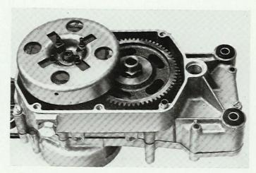
Hold the 2nd speed housing «C» with the tool 64766 and tighten the nut to 3÷4 kpm (in.lb. 0,168÷0,224) with torque wrench.
