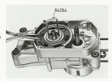
Remove the 10 crankcase screws from the right hand crankcase. Strike the ends of the crankshaft «A» and of the primary shaft «P» alternatively with a mallet until the two halves of the crankcase separate.
