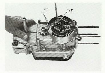
Using the tool 64753 and a 17 mm (.669") wrench remove the nut and the lock washer, then pull the sprocket from the shaft.
