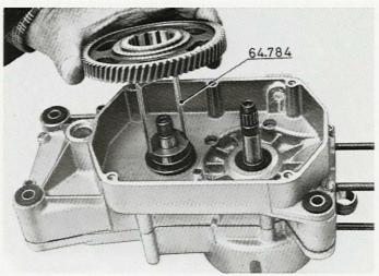
CAUTION: the freewheel hub shall be fitted so as to allow the 1st speed gear to turn free when rotated in the clockwise direction.
