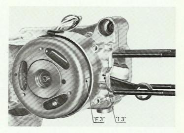
When satisfied that the gap is set correctly, fit the washer and tighten the fastening nut, using the tool 64781 and the 12 mm (.472'') socket previously used when dismantling.
