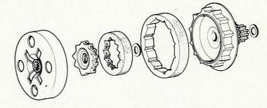
Hold the 2nd speed housing with the tool 64766 and tighten the nut with the tool 64783.
