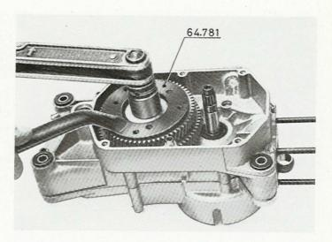
Remove the 2nd speed gear and then the 1st', while holding the catches with the tool 64784.
