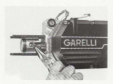
Remove the piston gudgeon pin using the extractor 64759 and a mallet, being careful to support the piston on the opposite side.
