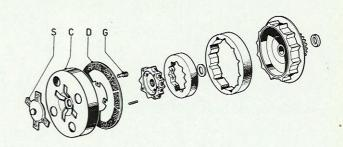
— When at the disc «D», place the 4 rubbers «G» in the corresponding holes. The rubbers ends should face towards the outer side of the engine and the thicker lined face of the disc towards the inner side of engine.
