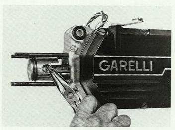
— Check that the crankcase upper face and the cylinder base are clean and free from burrs. Lightly grease a new gasket on both sides and lay it on the crankcase face. Oil the cylinder bore and the piston skirt. Lower the cylinder onto the piston with fingers compressing the rings into the bore. Make sure that the ends of the piston rings are properly fitted in position against the pegs of the ring grooves. Slide the cylinder along the 4 studs and fit it in place.
