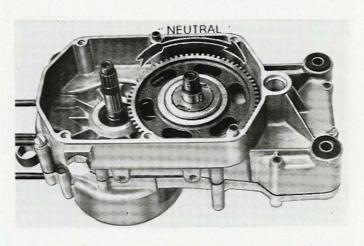
— With the tool 64781 and torque wrench tighten to  $8 \div 8,5$  kpm (in.lb.  $0,448 \div 0,476$ ) the nut fixing the gears on the primary shaft.
