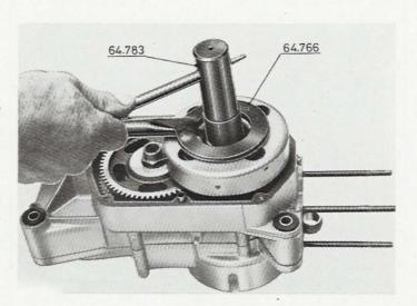
Take the assembly of two clutches complete with gears and slide it from the crankshaft.
