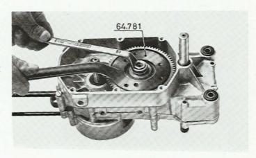
Use extractor tool 64757 and a 19 mm (.748") wrench to remove the gear.
