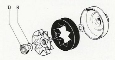
With the tool 64782 hold the clutch hub and tighten with the tool 64783 the nut «D» and washer «R» fixing it to the crankshaft.
