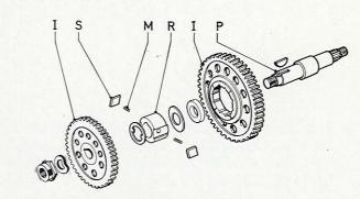
Place gears «I» and freewheel «R» on the primary shaft «P» as per illustration. Use the tool 64784 to hold in place the springs «M» and catches «S» when sliding the 1st speed gear on.
