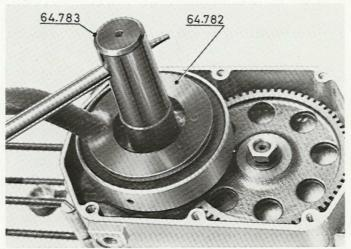
Assemble the starting assy. as illustrated. (This operation also applies to the single speed kickstarter models).
