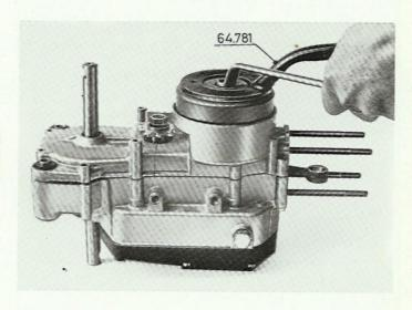
— Fit the chain gear and the two shim washers on the primary shaft, using the tool 64753 and a torque wrench tighten the nut to  $6 \div 6,5$  Kpm. (in.lb.  $0,336 \div 0,364$ ).
