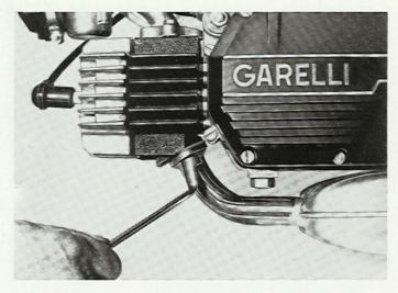
— On the pedals model only, disconnect the starting cable using a 17 mm (.669") open end wrench as illustrated.
