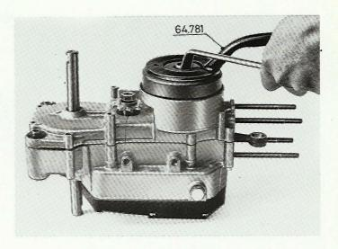
— Before using the extractor, the external threads and those of the center bolt should be lightly greased. Screw the extractor 64779 (for Bosch flywheels) or 64752 (for the others) into the threads of the flywheel, then turn the extractor center bolt in a clockwise direction to pull the flywheel off the taper; keep holding the rotor with the tool 64781.
