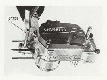
Using the tool 64781 to hold the flywheel, unscrew the flywheel retaining nut with a 12 mm (.472") socket. Remove the spring washer.
