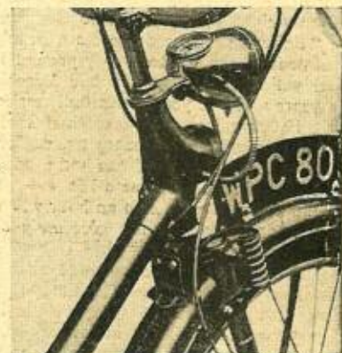
(Left) On the road the machine handled well. (Right) The speedometer is built into the head lamp; also seen is the neat anti-theft lock.
