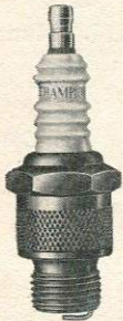
CHAMPION TYPE 7 Thread dia. 18\frac{m}{m} . Reach \frac{1}{2} ". Terminal A548. Hexagon 1". Gap setting normal .025".
