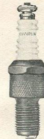
CHAMPION TYPE N3 Thread dia. 14\frac{m}{m} . Reach \frac{3}{4} ". Terminal A548. Hexagon \frac{13}{16} ". Gap setting normal .020".
