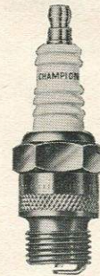
CHAMPION TYPE N5 Thread dia. 14\frac{m}{m} . Reach \frac{3}{4} ". Terminal A548. Hexagon \frac{13}{16} ". Gap setting normal .025".
