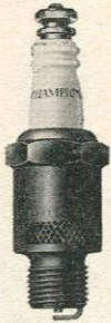
CHAMPION TYPE L-8 Thread dia. 14\frac{m}{m} . Reach \frac{1}{2} ". Terminal A548. Hexagon \frac{13}{16} ". Gap setting normal .020".
