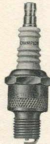
CHAMPION TYPE L-10 Thread dia. 14\frac{m}{m} . Reach \frac{1}{2} ". Terminal A548. Hexagon \frac{13}{16} ". Gap setting normal .025".
