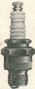
CHAMPION TYPE 8 Com. Thread dia. 18\frac{m}{m} . Reach \frac{1}{2} ". Terminal A146. Hexagon 1". Gap setting normal .020".
