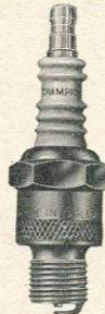
CHAMPION TYPE L-10S Thread dia. 14\frac{m}{m} . Reach \frac{1}{2} ". Terminal A548. Hexagon \frac{13}{16} ". Gap setting normal .025".
