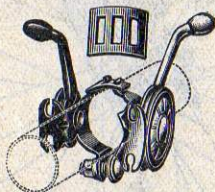
Showing "ROSA" lever coupling of c/w derailleur to "CYCLO" Gear Control.
