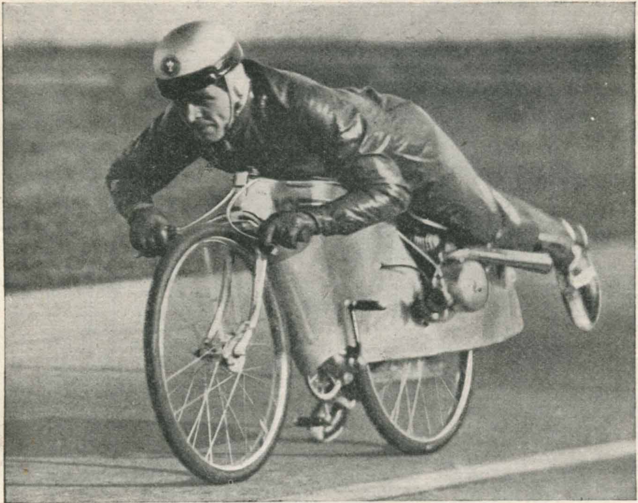
CLIP-ON RECORD: E. Dotterweich, of Germany, riding a cycle with a 38 c.c. Victoria motor attachment, broke the 50 c.c. class flying kilometre and flying mile records with a speed of 49 m.p.h. See page 426
