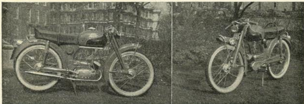
Clean motor cycle lines and a strong pressed steel frame characterise the Avanti
