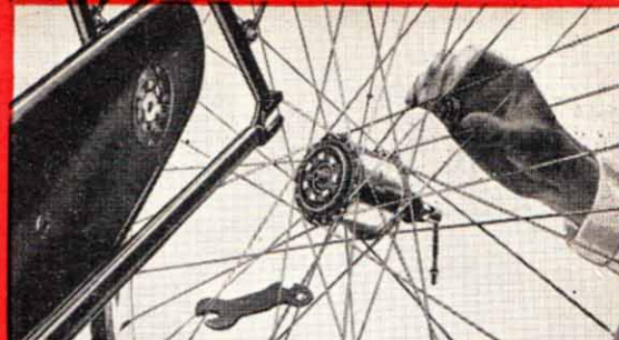
Quick Release 3-Speed Hub. 30 seconds to remove the wheel, leaving the chain and sprocket in position.
