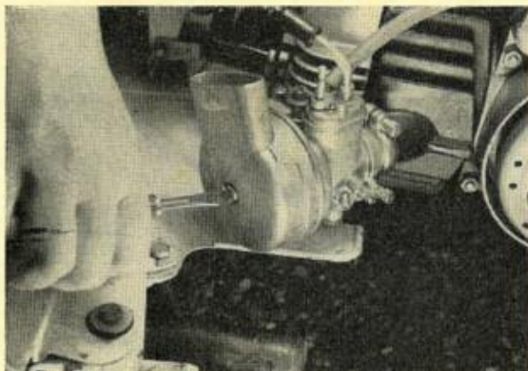
3. Dismantling air intake to reach the filter
