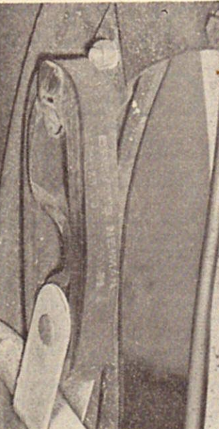
(Top left) The Gurtner carburetter filter nestles snugly in the frame. Note the petrol tap at the top left of the picture, and the engine springing.
