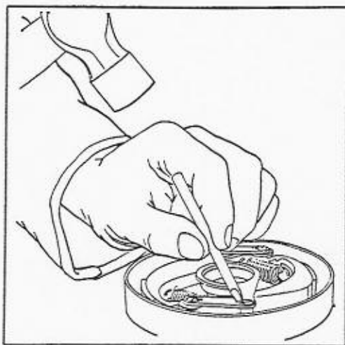
Fig. 18 Locking countersunk screws
