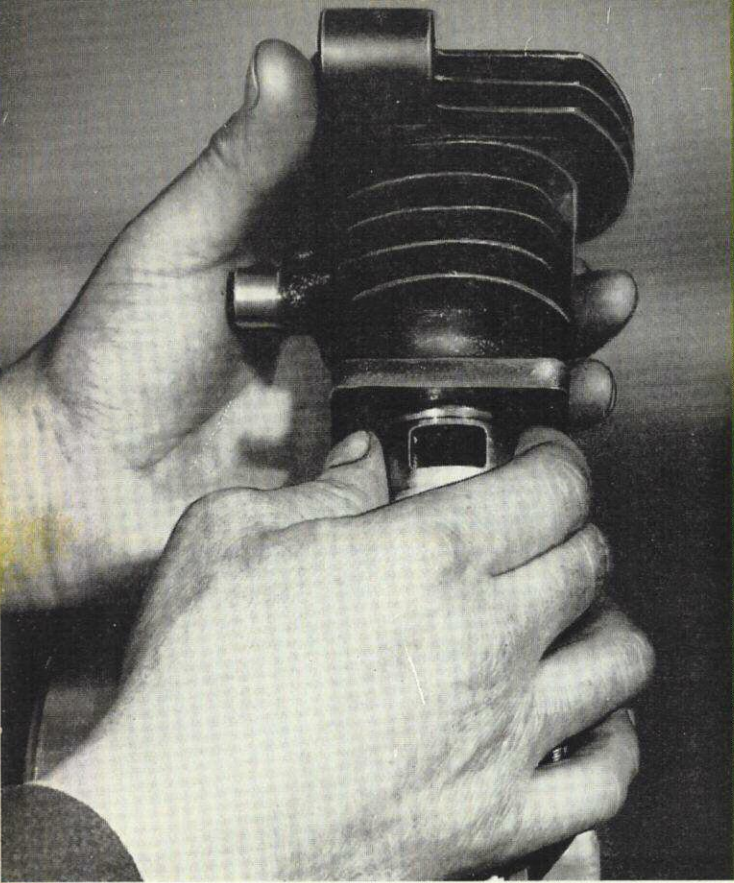
FIG. 19 Fitting piston into cylinder.
