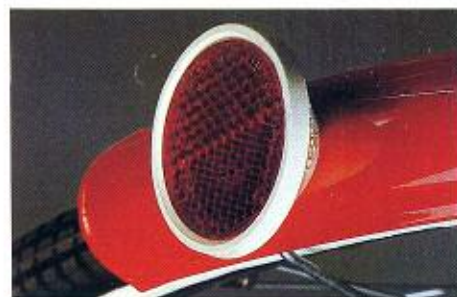
Large diameter, rear mudguard-mounted safety reflector.
