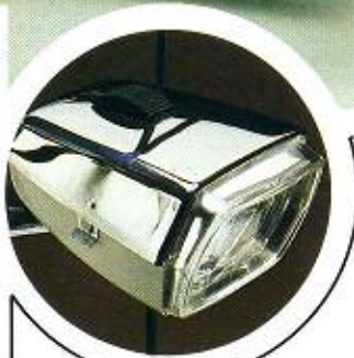
Sturmey-Archer combined "Dynohub" lighting equipment and 3-speed gear is available as an optional extra on Wayfarer.
