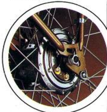
Sturme-Archer "Dynohub" lighting equipment with a combined 3-speed gear is an optional extra on these models.
