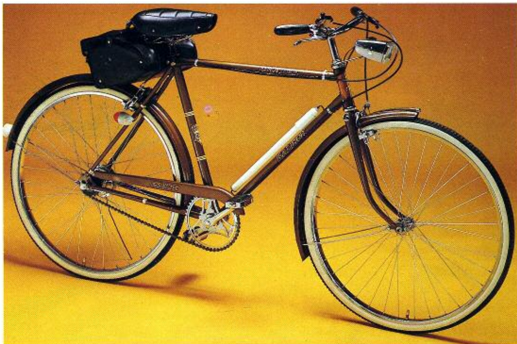
Sturme-Archer "Dynohub" lighting equipment with a combined 3-speed gear is an optional extra on these models.
