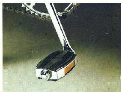
Pedal reflectors – the pedal movement creates immediate attention as headlamps are reflected.
