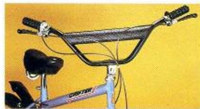
Stylish handlebars on Grifter have special facia panel in foam plastic with reinforcing steel tie-bar.
