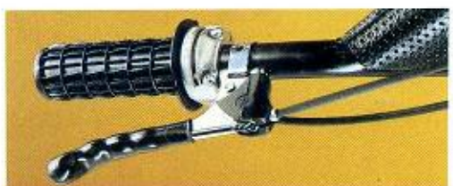
Sturmey-Archer twist grip control operates the 3-speed gear from the handlebars.
