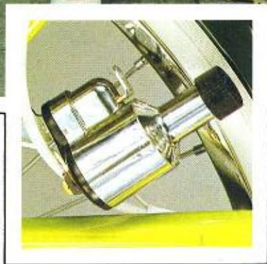
Tyre-driven dynamo lighting set – an optional extra on Nova.
