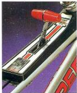
Gear Change Console. A snap-action movement to change the Sturmey-Archer 3-speed gear – smooth and positive.
