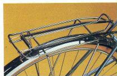
Chrome rear carrier with expanding retention grip.
