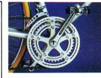
Raleigh branded alloy chainset of cotterless design with chainring guard.
