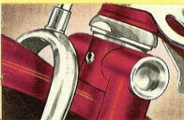
RALEIGH HOODED LEVERS. Fitted to all models with our calliper brakes, comfortable to operate due to absence of external bolt heads or nuts.
