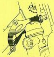
RALEIGH BELL CRANK. Careful design, combined with extreme neatness, provide a smooth and very efficient rear centre pull roller lever brake.
