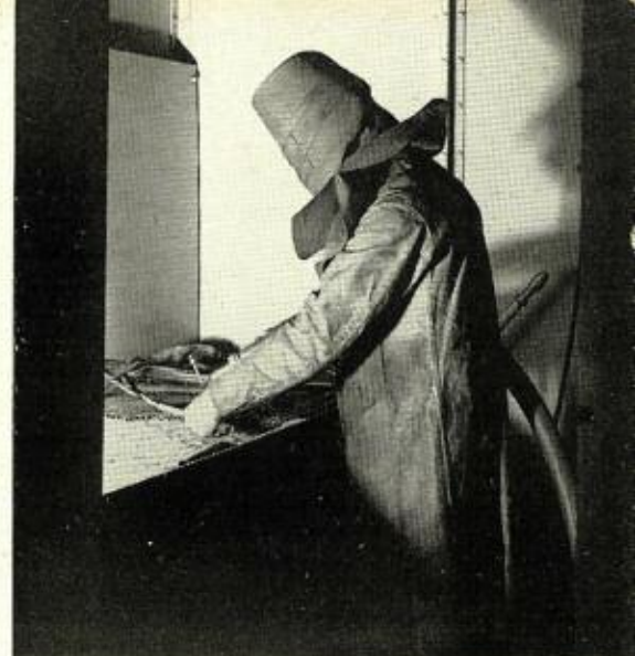
A workman wearing protective clothing engaged in a cubicle of the shot blasting departments
