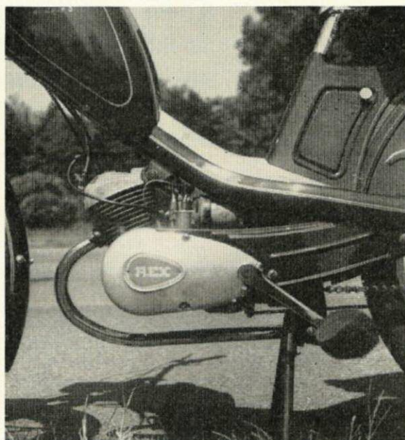
The new three-speed unit differs slightly in appearance from the two-speed model but the rest of the machine is the same. Note the very low saddle position available and the easy accessibility of all maintenance points
