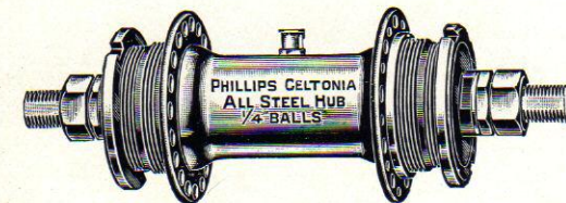
No. 43.—Celtonia Rear Racing Hub. 1½" Chain line. Without Gear Case Clearance Screwed both sides to take Cog and Lock Nut or Free Wheel. Flatted for use in 5/16" Quick Release Fork Ends.
