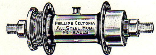
No. 40.—Celtonia Rear Hub. 1½" Chain line. Without Gear Case Clearance Screwed one side only for Cog and Lock Nut or for Free Wheel. Flatted for use in 5/16" Quick Release Fork Ends.
