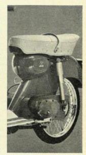
APPRECIATE: Oildamped swinging arm; full shielding round rear wheel; long broad dualseat for big man comfort.
