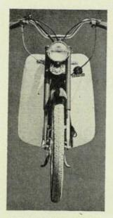
STURDY telescopic forks; effective 17 watt headlamp; electrical horn; adjustable handlebars; powerful brakes.
