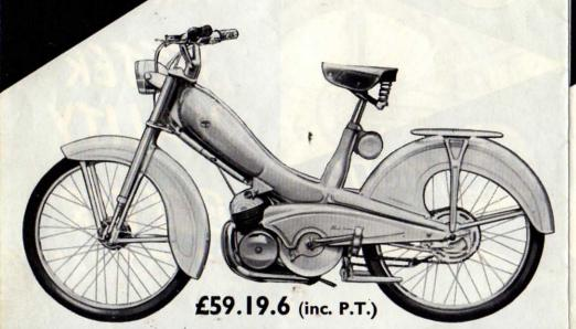
Engine: 49 c.c. high efficiency; chrome lined cylinder with flat-top piston; 1.35 b.h.p. at 3,400 r.p.m.
