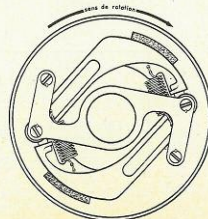
BG clutch : view of the flyweights
