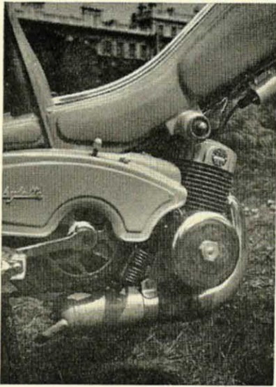
Note the large rubber-bushed engine bearer and tension spring. The H.T. coil can be seen top right
