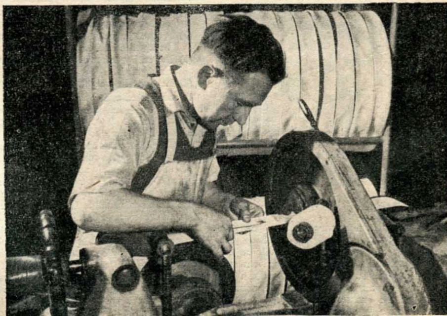
(Above) Testing a strand of cotton cord used in making tyre fabric. It must have tensile strength but little stretch. (Below) Building a cycle tyre casing on a semi-automatic machine.
