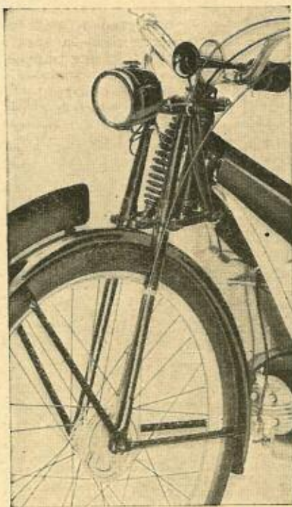
Arrangement of the new central-spring front forks
