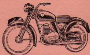
MODEL L15 - CADET 150 First frame number AL15/3082 Villiers 147 cc. Mk. 30C engine
