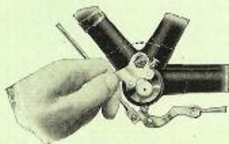
The JAMES Bottom Bracket and adjustment. To adjust, use pegged spanner provided, and turn gently to right hand as shown by arrow indication
