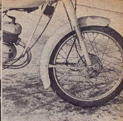
The front brake proved a good stopper. Other cable shown is the drive to the speedometer
