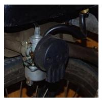
convenient were they the other way. There is a little sink in the bottom of the float chamber with a drain screw, this conveniently collects the dirt from my fuel tank. There is a spring loaded throttle stop screw.
